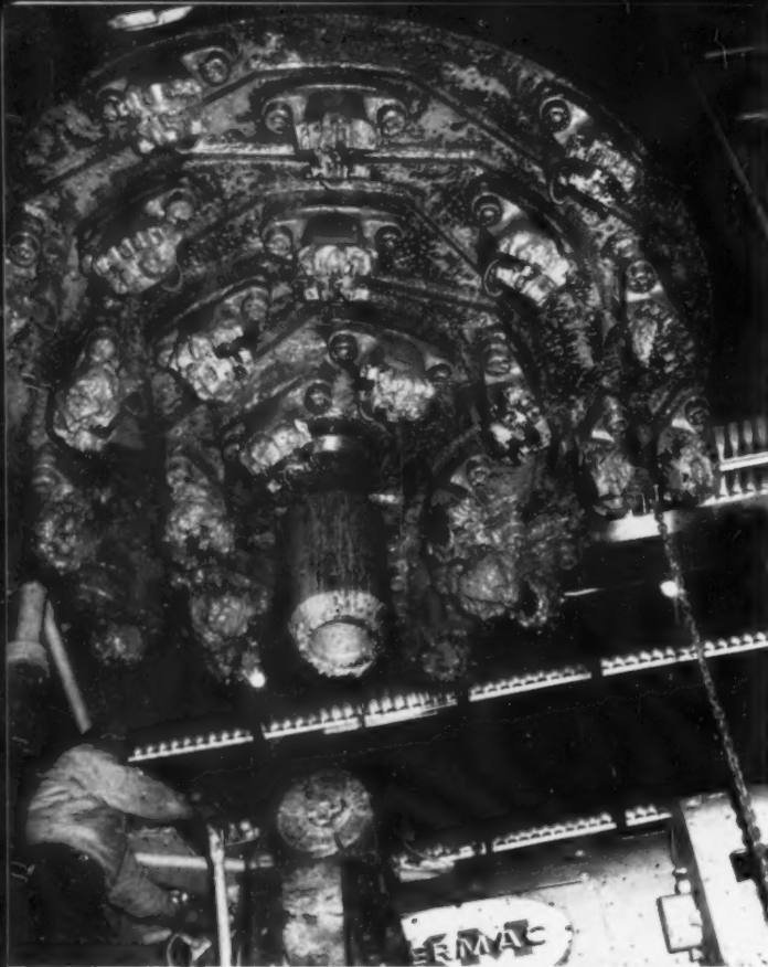
BIG BIT is pulled out of shaft. Drilling face shows 28 Hughes rolling cutters in seven stages. Stinger bit has been uncoupled.
